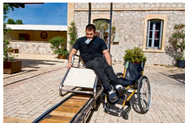
The Seatrac user will leave the wheelchair further away from the water and cover the distance to the sea using the device. Small photo on the left: view of the device assembly. The structure is not permanent and it is environmentally friendly, as it runs on solar power
