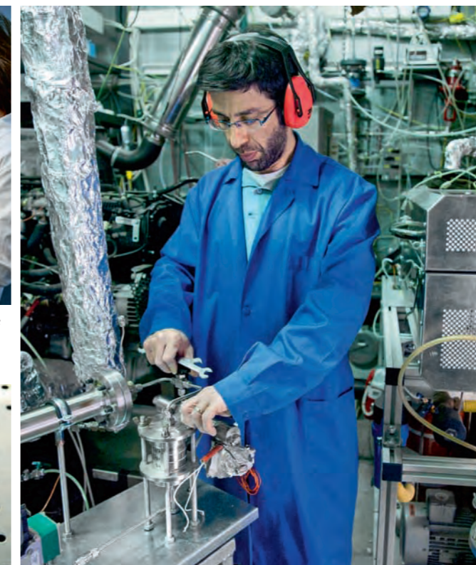
Mr Akritudis putting together the Impactor of the Selective Particle Size (SPS) sampler.
