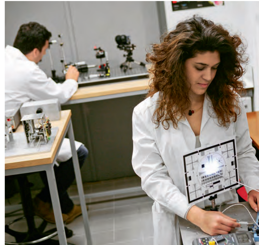
Quality control laboratory testing of the spectral hyper-vision endoscope.
