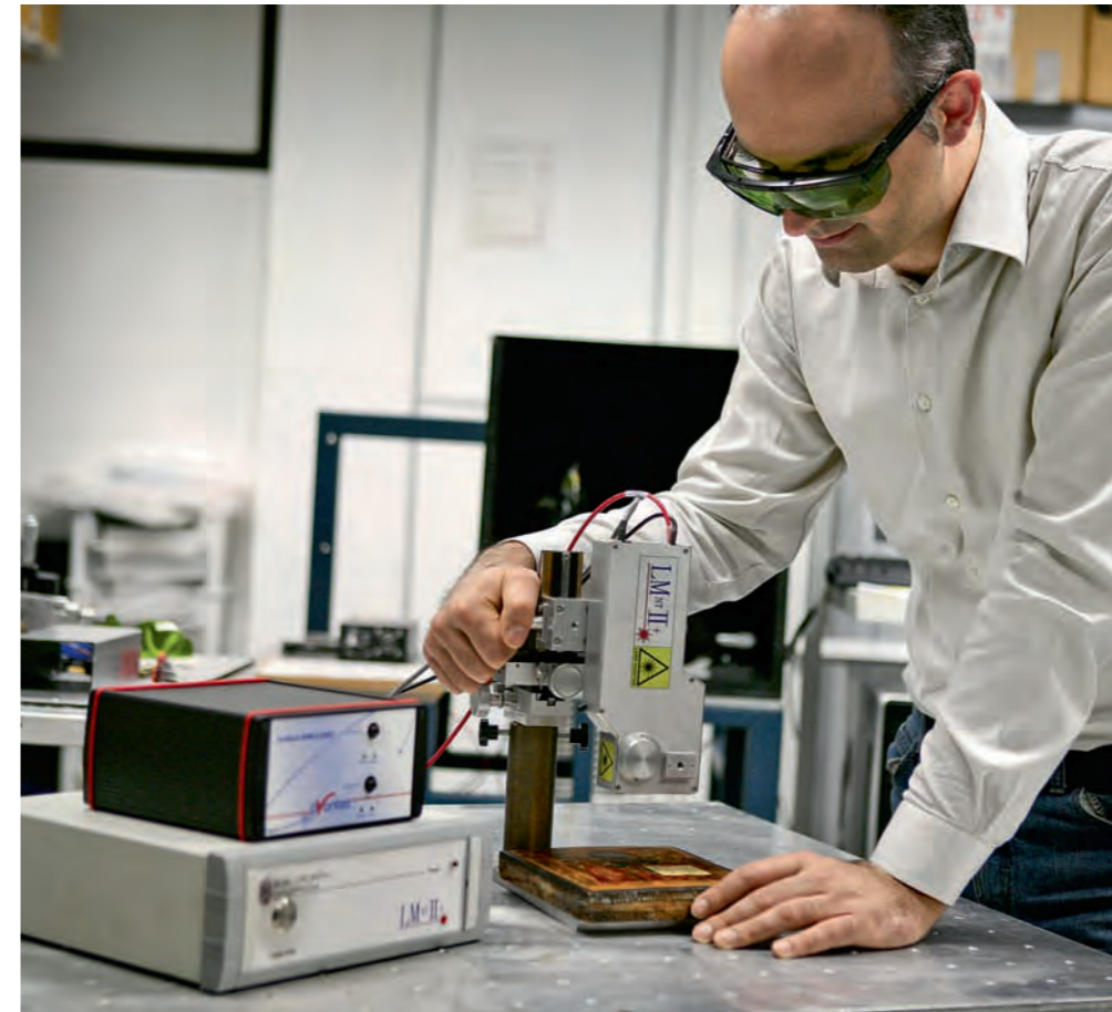
In just a few seconds, the device not only identifies the elemental composition of any solid material, but also determines the quantity of each chemical element contained in the sample.
