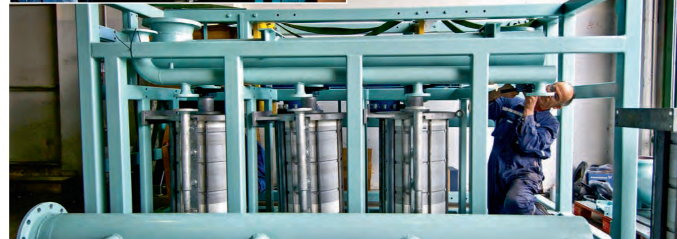
Final assembly of an ERMA FIRST BWTS 400. The system is destined for a Greek-owned ship under construction in a South Korean shipyard.
