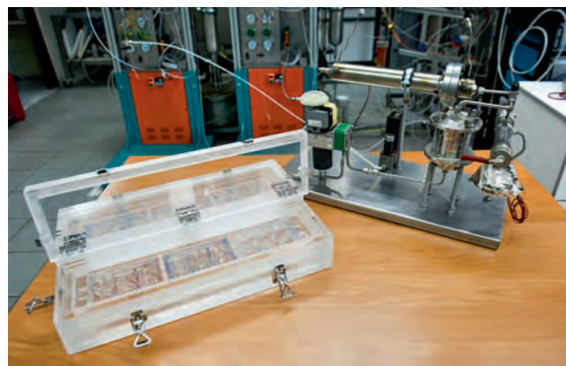
Multiculture Exposure Chamber (MEC)(on the left) and Selective Particle Size (SPS) sampler (on the right).
