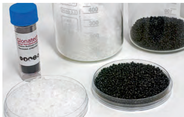
Nanostructured carbon in the form of a composite material with a polymer.
