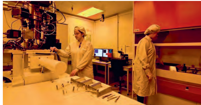
Located in the clean room of the Microelectronics Department, the unique electron beam lithography infrastructure in Greece shapes matter in dimensions below 10 nanometres.
