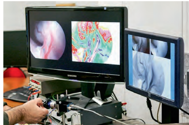
In addition to the magnified coloured image of the area scanned by the endoscope (on the left), a spectral map will be displayed on the device monitor (on the right), where cancer cells will appear in red to stand out.
