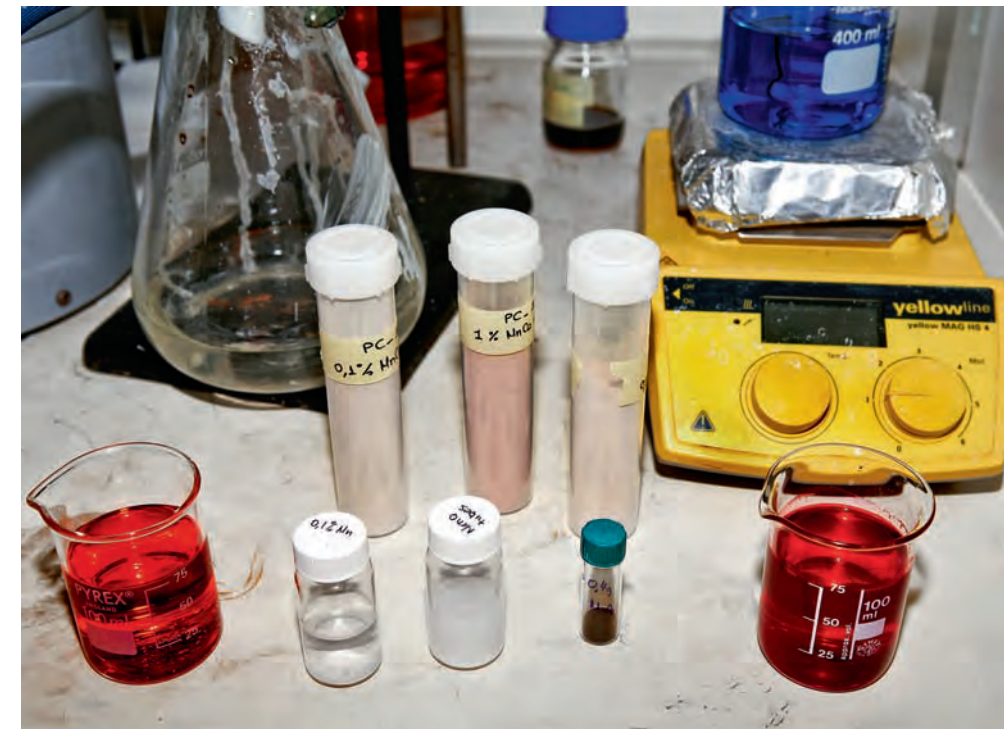
Powders of photocatalytic solids with varying manganese content during the first tests for decomposing pollutants.
