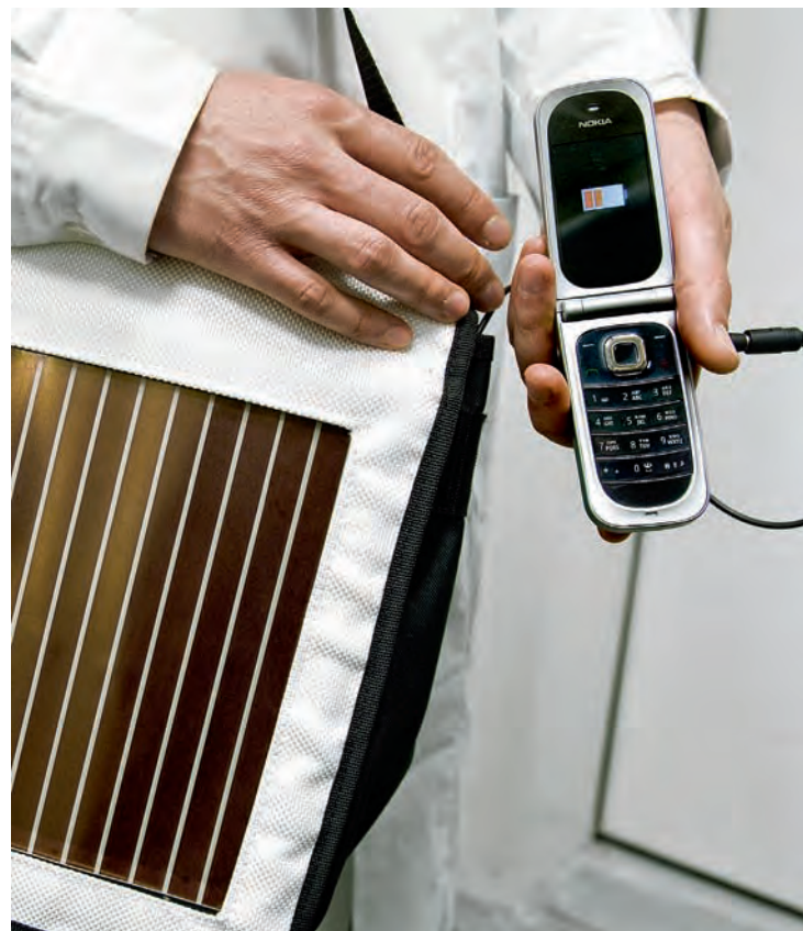
Above: The first complete application of the innovation. A handbag covered with flexible organic photovoltaics produces enough electricity to charge a mobile phone. Right: Professor Stergios Logothetidis (first right) with members of the scientific team.
