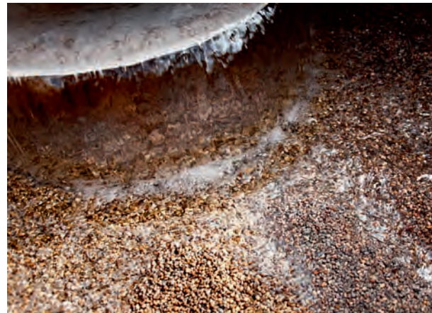
The water cascades from the interior of the filter onto the surface of silicic gravel. Right: Professor Dimitrios Vayenas and his associate, Dr Athanasia Tekerlekopoulou, with their innovation in the background.
