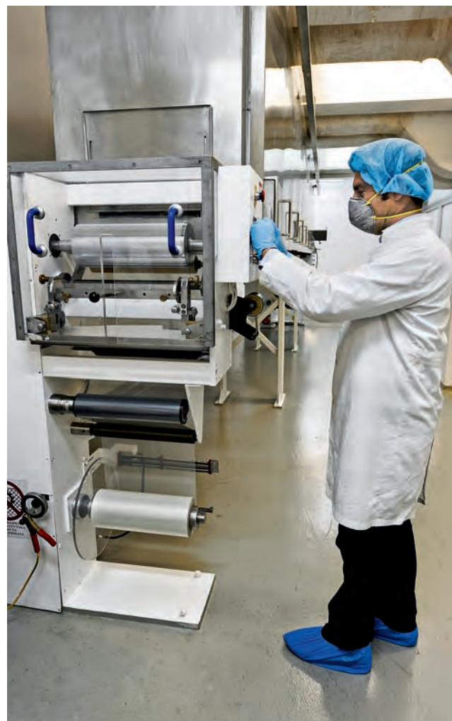
Main production line: coating, drying, creating a mother roll.
