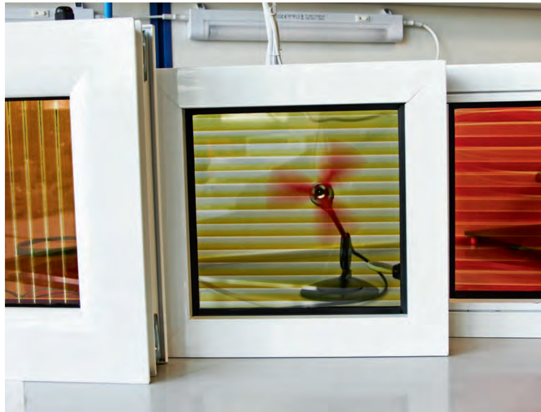
Left: Experimental application of the innovation. Glass panes fitted on small windows produce enough power to keep a small fan running constantly. Below: Dr Nikolaos Kanopoulos has extensive experience in semiconductor and solar panel technology. After 28 years in the USA, he created a 100% Greek innovation. Right: Measuring and testing at Brite Solar's laboratory, housed within the Patras Science Park.
