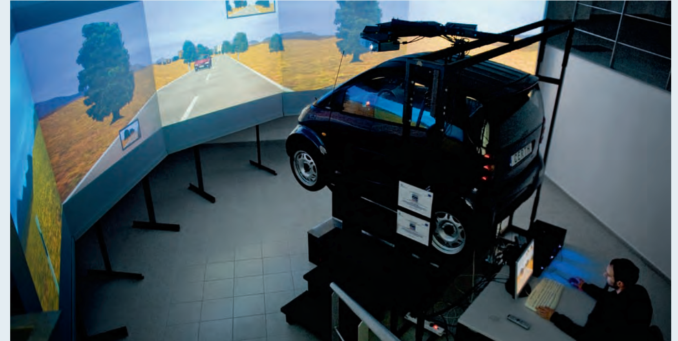
CERTH’s Hellenic Institute of Transport has the largest driving simulator in Southeast Europe. The simulator is a piece of research equipment that can be used to conduct a series of tests and experiments on driving behaviour in various conditions, to test advanced driver assistance systems (ADAS), and to analyse the impact of using such systems on driving behaviour and, by extension, road safety.
