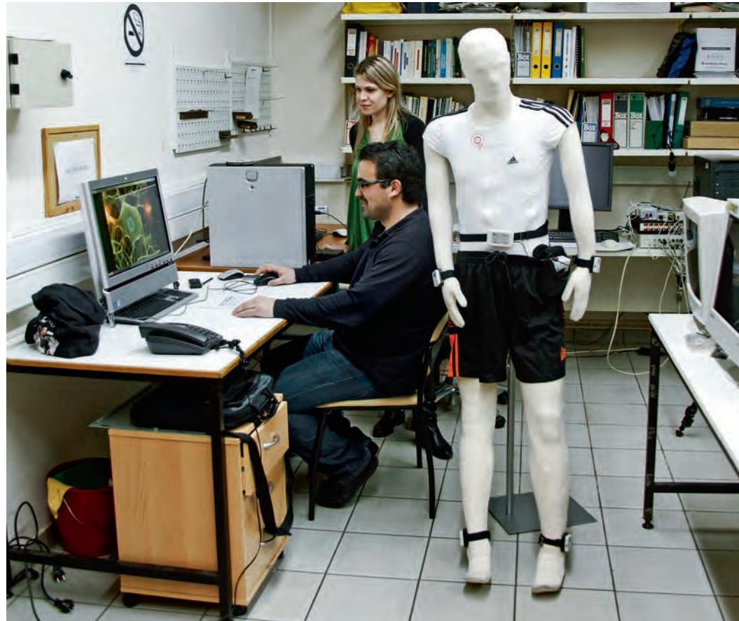
In the laboratory, Professor Fotiadis' associates are testing the Perform system on a dummy patient. The five sensors can be seen on the hands, the legs and around the waist.
