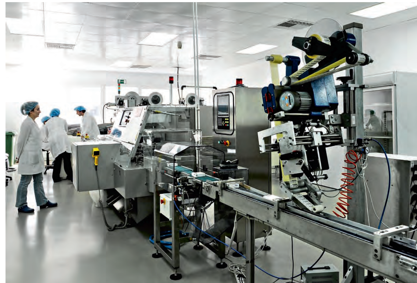
The film is placed in individual envelopes through a fully automated packaging line.
