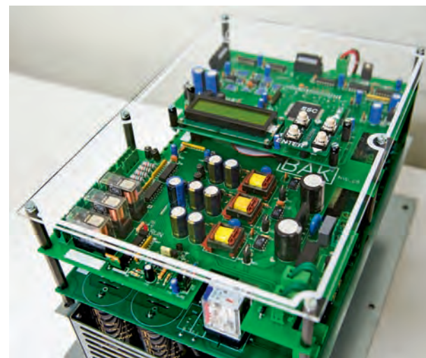
The integrated self-tuning inverter. Right: Nikos Michalodimitrakis (front) and Periklis Neofotistos with colleagues in the company's laboratory.
